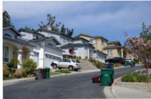
In this hillside subdivision, building height and bulk is minimized through horizontal and vertical setbacks and step-backs. (Guideline B-4)
